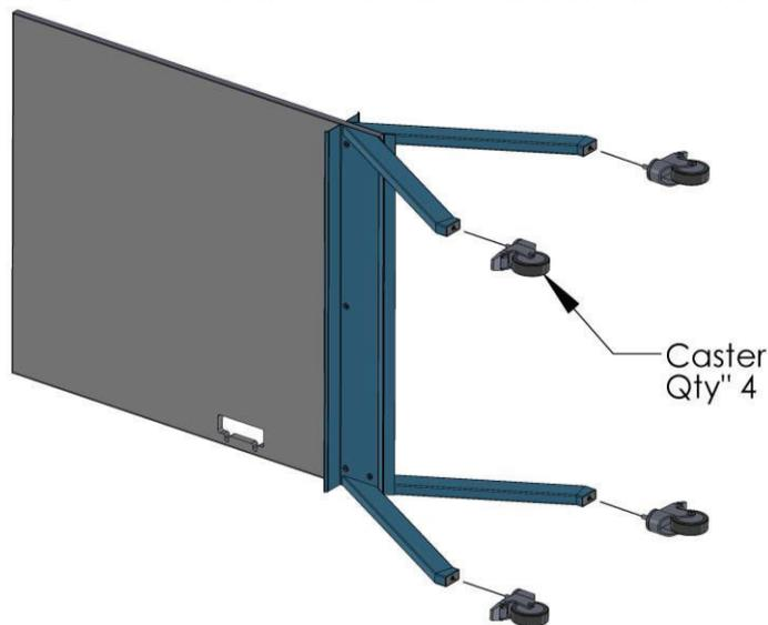
**Step 3:** Place the whiteboard in the upright position which then will auto-level itself. Now fully tighten the connector bolts; **two individuals should perform this step, in order to prevent injury**. Install the handle using the supplied plastite screws.
